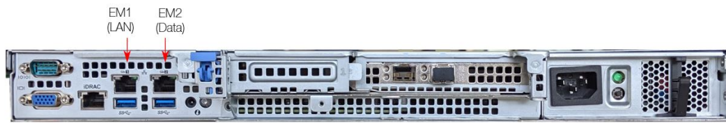
Figure 4.6: PILATUS3 R 200K-A detector control unit as seen from the back.
