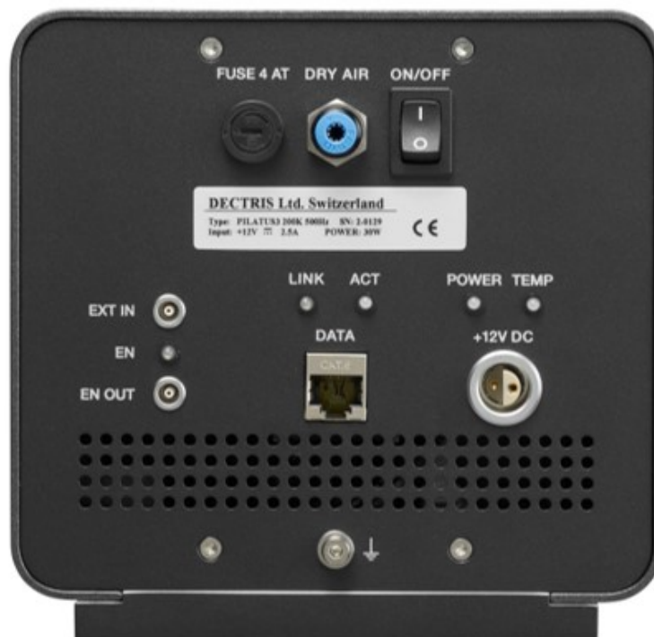
Figure 4.4: The PILATUS3 X 200K-A detector (back view)
